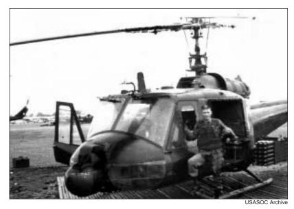
A crew chief from the 281st stands beside a UH-1C "Hog Frog" that is equipped with 2.75-inch rocket pods and a "chin-mounted" 40 mm grenade launcher.
