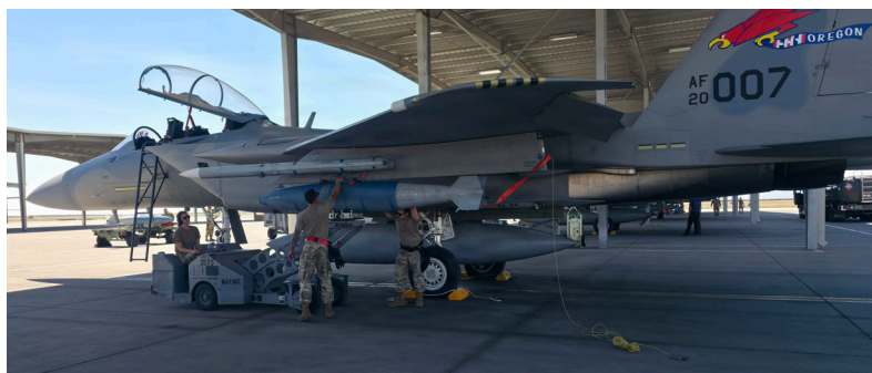
A BDU-56 "bomb" is loaded onto an F-15 EX Eagle II aircraft assigned to the 142nd Wing during a training mission at Mountain Home Air Force Base, in May 2026.
