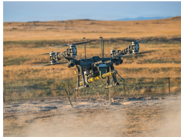
A Lorica Technologies Inc. Mule 28 unmanned aerial system carries a live, primed M1A3 Bangalore torpedo toward a concertina wire obstacle moments before release on June 22, 2026.
