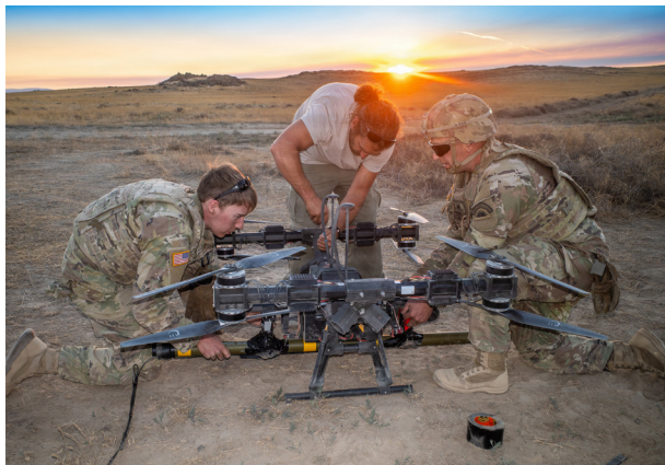
(L-R) Capt. Samuel Cushing, 741st BEB, Austin Hansen, director of manufacturing for Lorica Technologies Inc., and 1st Lt. Andrew Lucas, of the battalion's S-3 section, attach a live M1A3 Bangalore torpedo to a Lorica Mule 28 unmanned aerial system.
