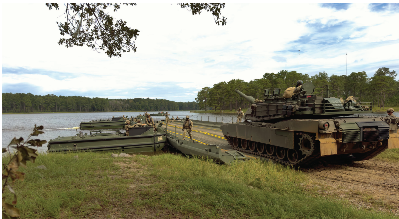
Figure 3. A 3rd Infantry Division M1A2 SEPv3 Abrams main battle tank moves onto a barge made of several bridge segments during a wet-gap crossing exercise in Fort Stewart’s Pineview Lake. (U.S. Army photo by Kevin Larson)
