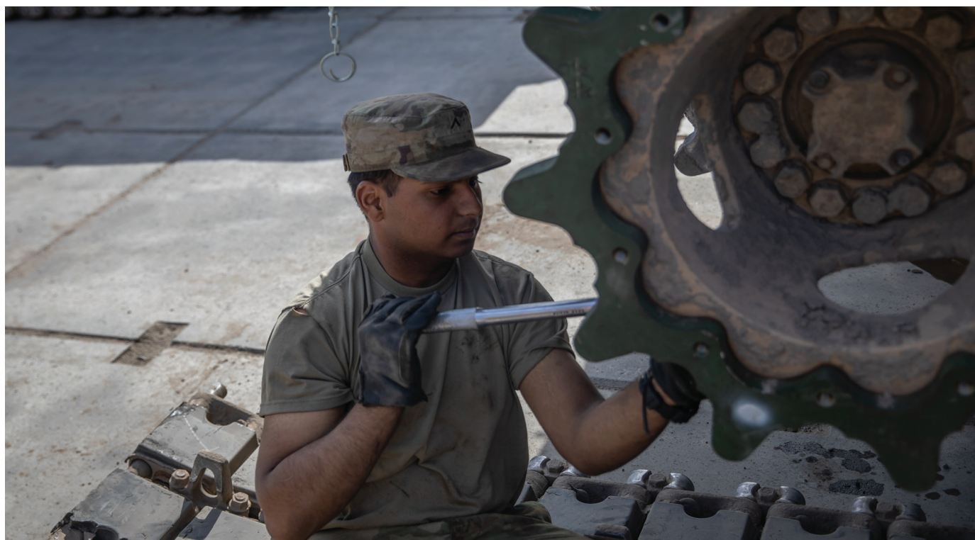
Figure 1. PVT Pragyan Poudel, assigned to Alpha Company, 2nd Battalion, 70th Armor Regiment, 2nd Armored Brigade Combat Team, 1st Infantry Division supporting the 4th Infantry Division, installs a new sprocket onto an M1 Abrams tank during maintenance, at Nowa Deba Training Area, Poland, May 11, 2023. (U.S. Army photo by PFC Jason Klaer)
