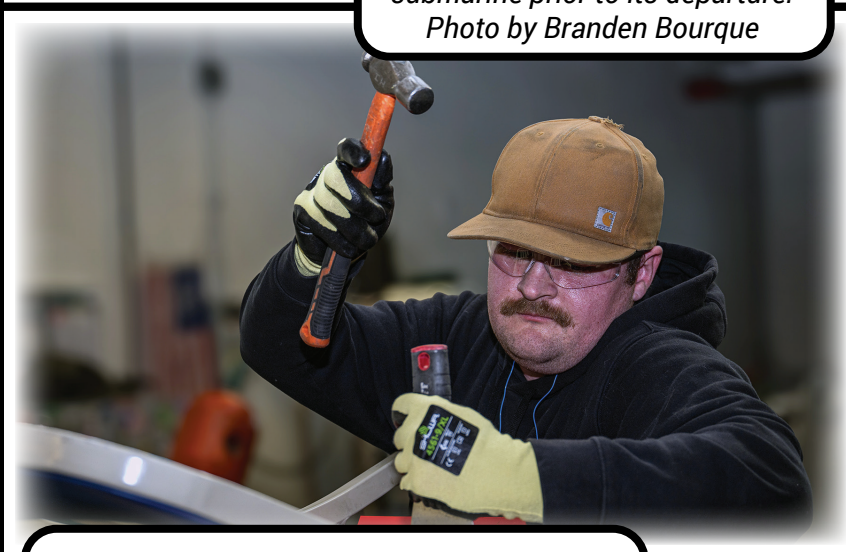
Sheet Metal Mechanic Ryan Pennell prepares a chair's steel frame for powder coating. Photo by Branden Bourque
