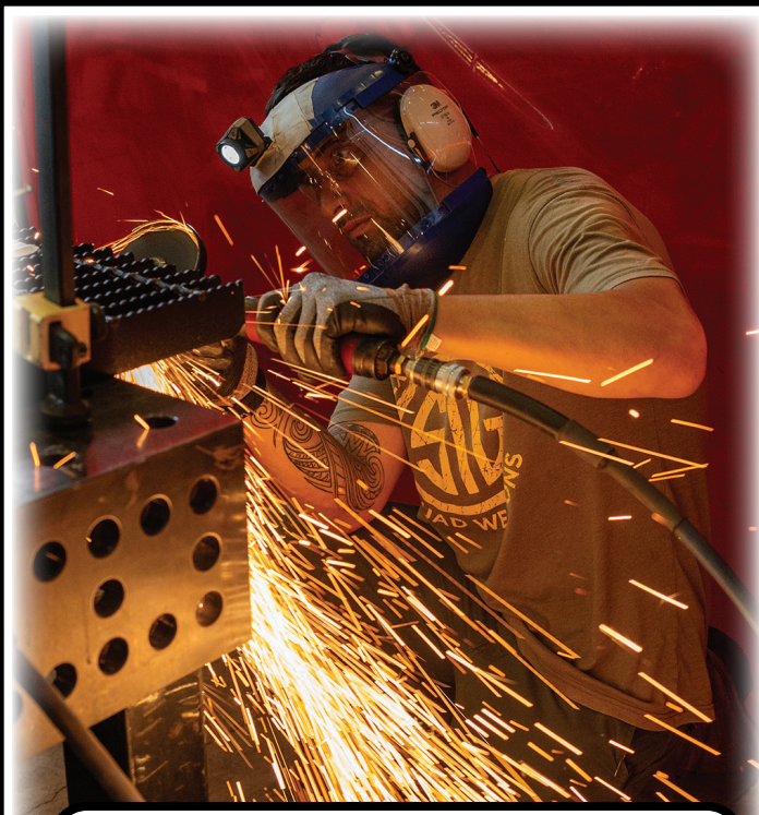
Shipfitter Peter Morris uses an angle grinder to touch up a steel grate. Photo by Neil Boorjian
