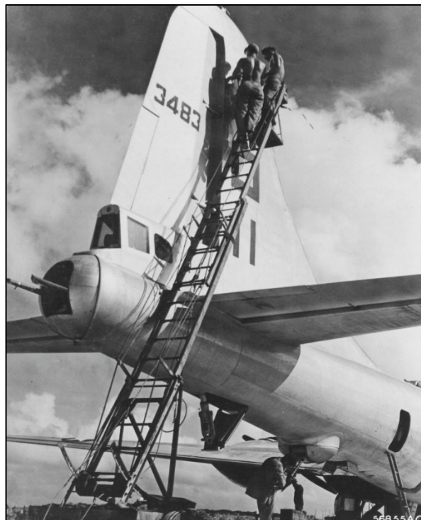
Figure 4: Mechanics repair a bullet hole in the vertical stabilizer in a Marianas-based Boeing B-29 suffered during a raid on an aircraft factory near Kobe, Japan.
