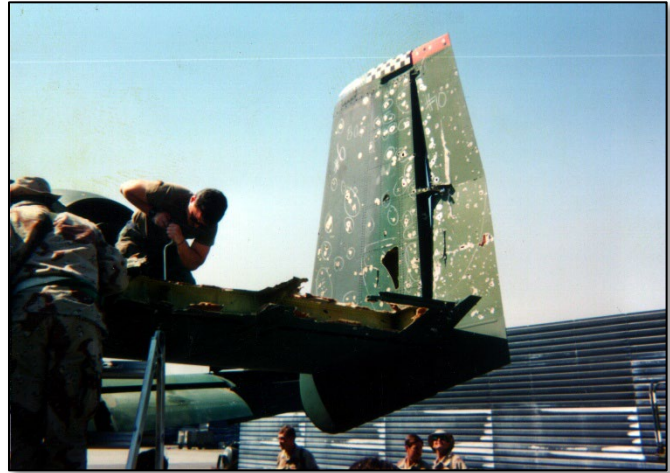
Figure 7: Fairchild Republic A-10 Thunderbolt II being repaired by ABDR teams during Operation DESERT STORM.
