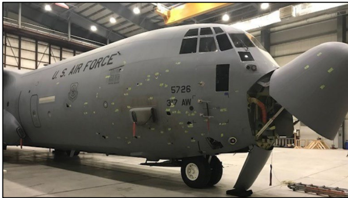
Figure 10: An ABDR repaired Lockheed Martin C-130J Super Hercules that suffered severe shrapnel damage from a mortar strike at Bagram AB, Afghanistan while it was taxiing out for take-off.
