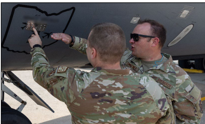
Figure 12: Members of the 76th Aircraft Maintenance Group's Expeditionary Depot Maintenance Flight inspect repairs completed by the ABDR team, allowing the KC-135 to fly back to Tinker to complete repairs.
