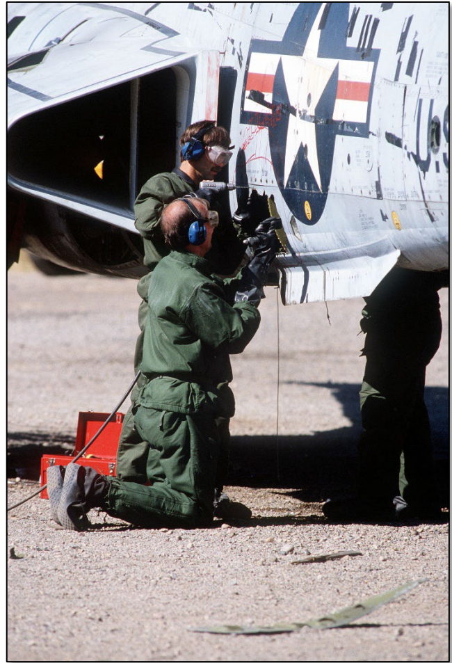
Figure 6: 2952 CLSS crews from Ogden ALC repair an F-101 during an ABDR exercise.
