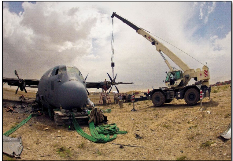
Figure 9: ABDR members from AFMC deployed to the 379th Air Expeditionary Wing in 2013 forward deploy to a forward operating base in Afghanistan for reclamation and demilitarization of a C-130J Super Hercules, recovering 250 components totaling more than $20 million.
