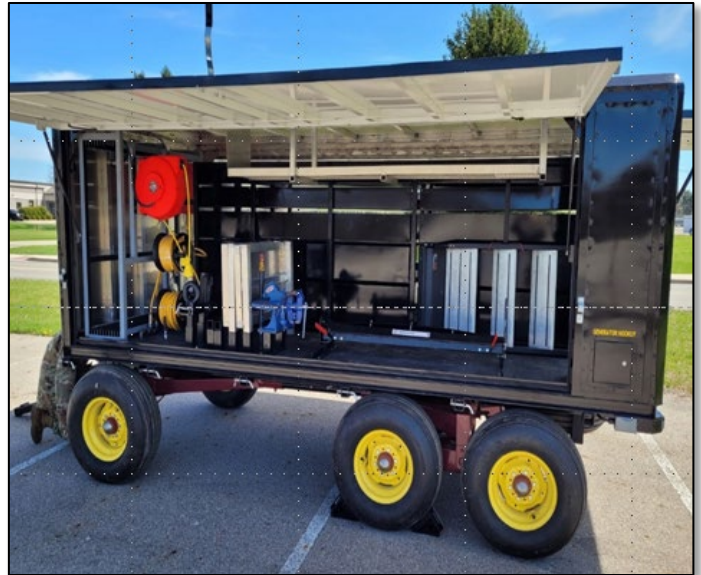
Figure 11: ABDR War Wagon, a concept dating back to the 1940s, contains materiel to support initial repair of damaged airframes.
