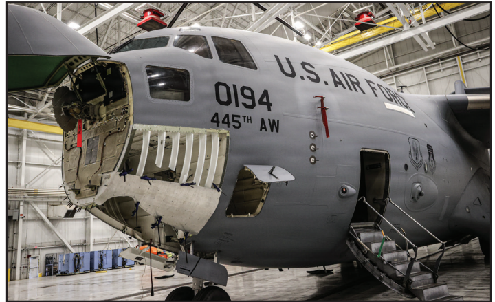
The newly formed nose panel undergoes an initial fit check on a C-17 Globemaster III at Wright-Patterson Air Force Base, April 20, 2026. (Photo by Casey Tromp)
