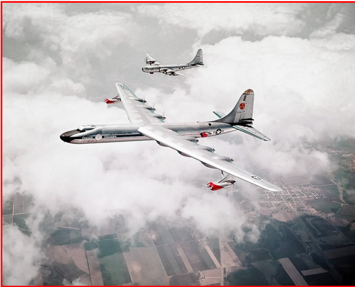
The NB-36H with a B-50 in 1955, the only aircraft to carry a nuclear reactor.
