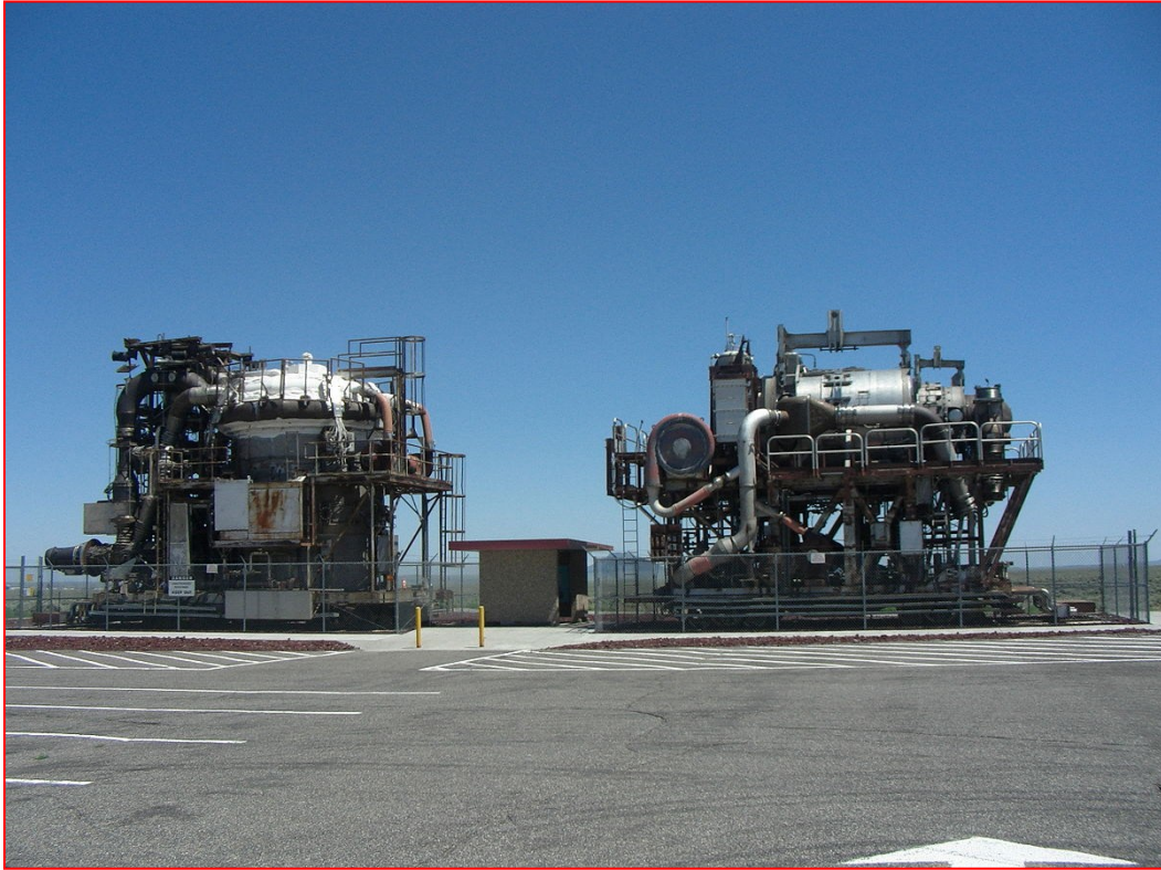
HTRE-3, left, and HTRE-2, right, now on display at the Idaho National Laboratory near Arco, Idaho. HTRE-2 was the converted HTRE-1. HTRE-1 or “Heater One” demonstrated the principle of nuclear-powered turbojet engines.
