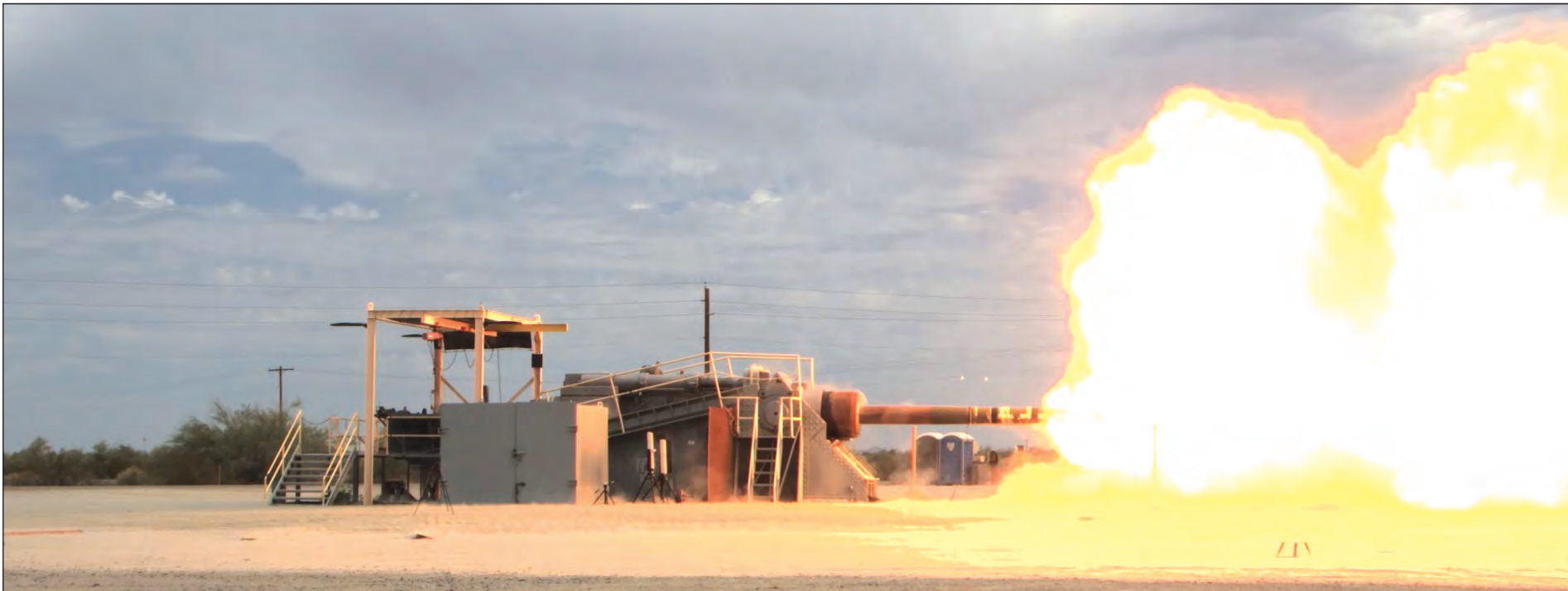
Yuma Proving Ground (YPG) successfully supported a full-scale, live-fire hypersonic warhead test out of a cannon base test system. The initiative began two years ago as a bold concept: utilizing a cannon-based approach to fire hypersonic warheads to conduct lethality assessments. (U.S. Army Photo)
