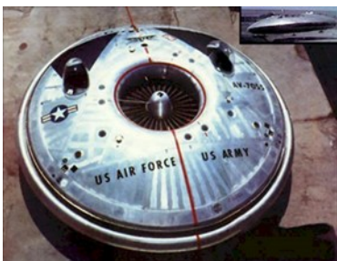
Avrocar, a vertical take-off and landing aircraft developed by the Air Force and Army.
