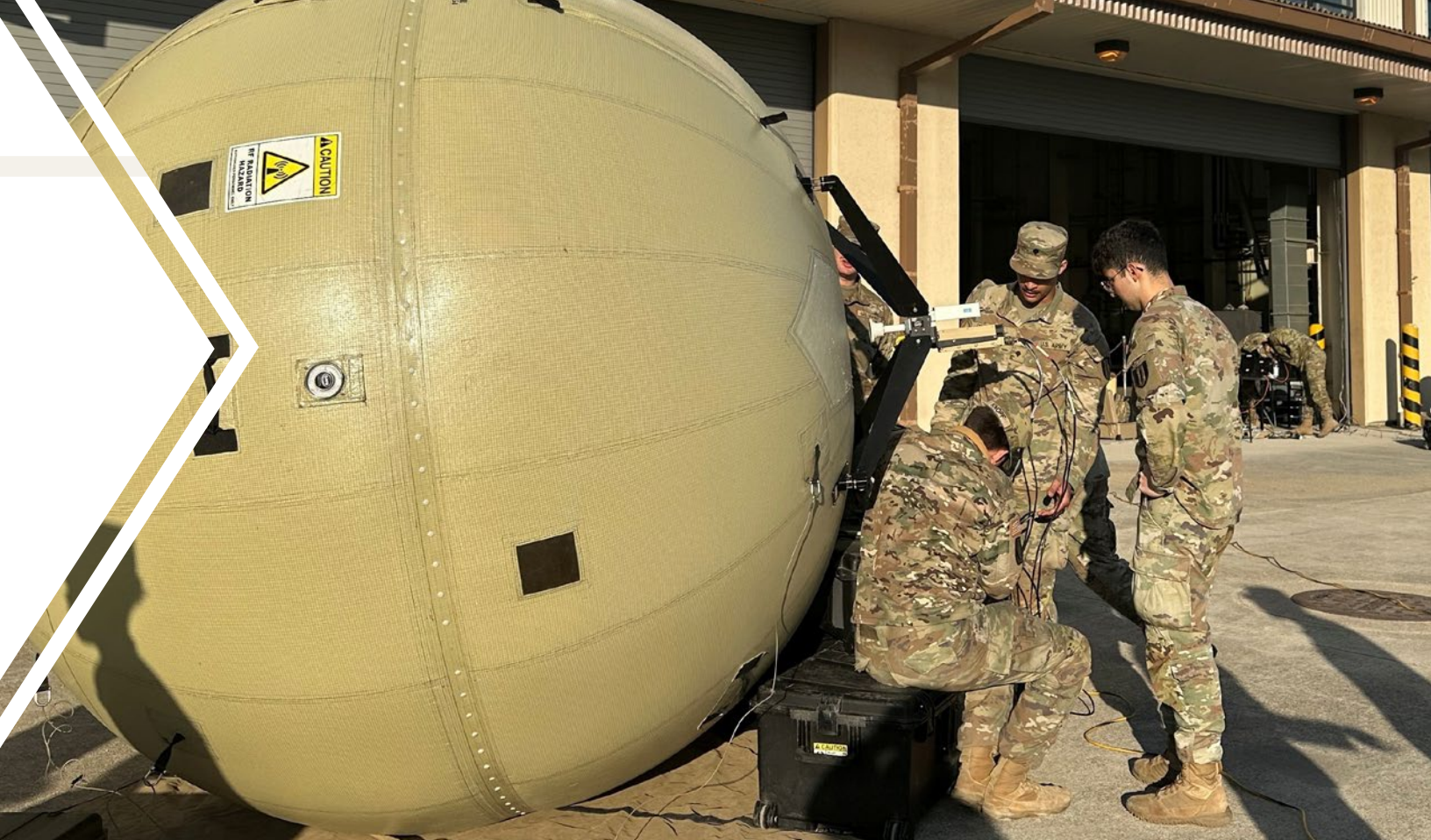
Above: U.S. Army Soldiers assigned to the 304th Expeditionary Signal Battalion - Enhanced install a 3D-printed replacement component on an AN/TSC-233 Transportable Tactical Command Communications system. The repair demonstrates how additive manufacturing can improve readiness by reducing maintenance costs and turnaround times. (U.S. Army photo courtesy of Maj. Karl McKeeth)
