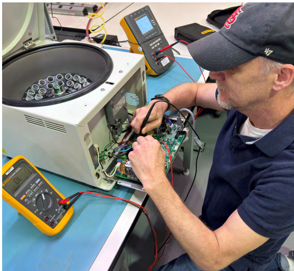
Electronics Technician Dave Williams uses a multimeter to diagnose an issue with a centrifuge machine at U.S. Army Medical Logistics Command's Medical Maintenance Operations Division at Tobyhanna Army Depot, Pennsylvania. Williams is part of a two-person team at MMOD-PA that supports the Military Entrance Processing Station, or MEPS, program, providing essential medical screening equipment for new recruits as they join the armed services. (Courtesy photos)
