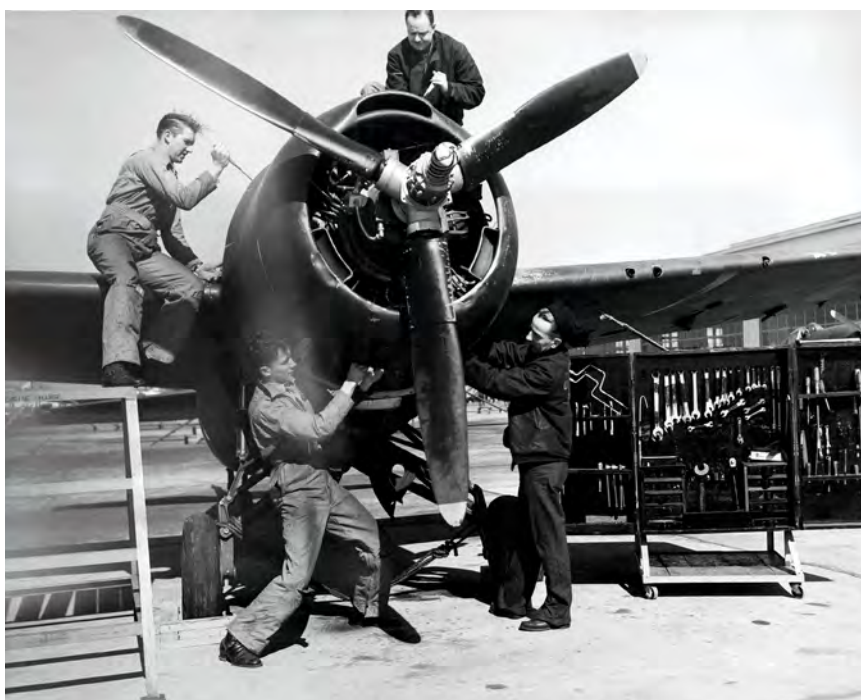
Trainees perform 30-hour check on “live” aircraft at Naval Air Technical Training Center, Naval Air Station Memphis. Practical learning enabled trainees to quickly obtain the skills necessary for deployment. (NHHC, L 39-18.01.01)
