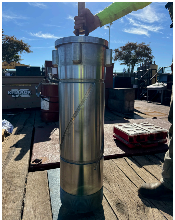
Newly regrooved gudgeon hinge pin. The spiral cuts allows the grease to be distributed around the entire pin and not only on the front side. Photo by Mike Barry
