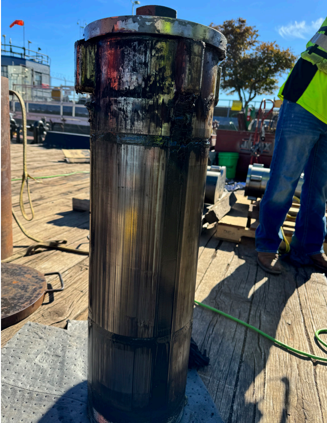
A worn hinge pin showcasing extraneous wear and tear due to a lack of grease being moved across the pin. Photo by Mike Barry
