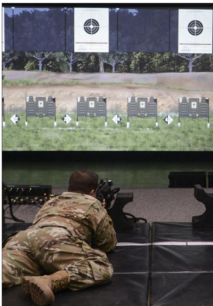
The Engagement Skills Trainer II (EST II) is designed to assist and improve the basic fundamentals of marksmanship, as well as collective and escalation of force training before going to a live-fire range. (Photo Credit: U.S. Army)
