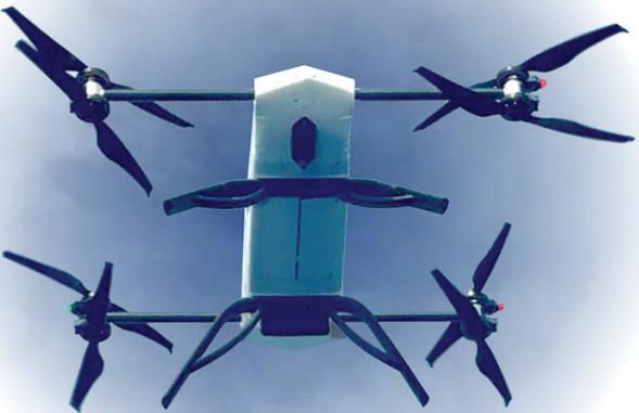
UAS platforms such as this Blueflite 461 can deliver emergency supplies, relay location data, and map complex environments with minimal risk to human life. Auxiliary photo by Cara Templeton.
