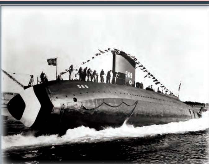
The USS Albacore (AGSS 569), launched from PNSY on September 1, 1953. The Albacore's evolutionary teardrop-shaped hull design became the prototype for the Navy's nuclear powered submarine force.
