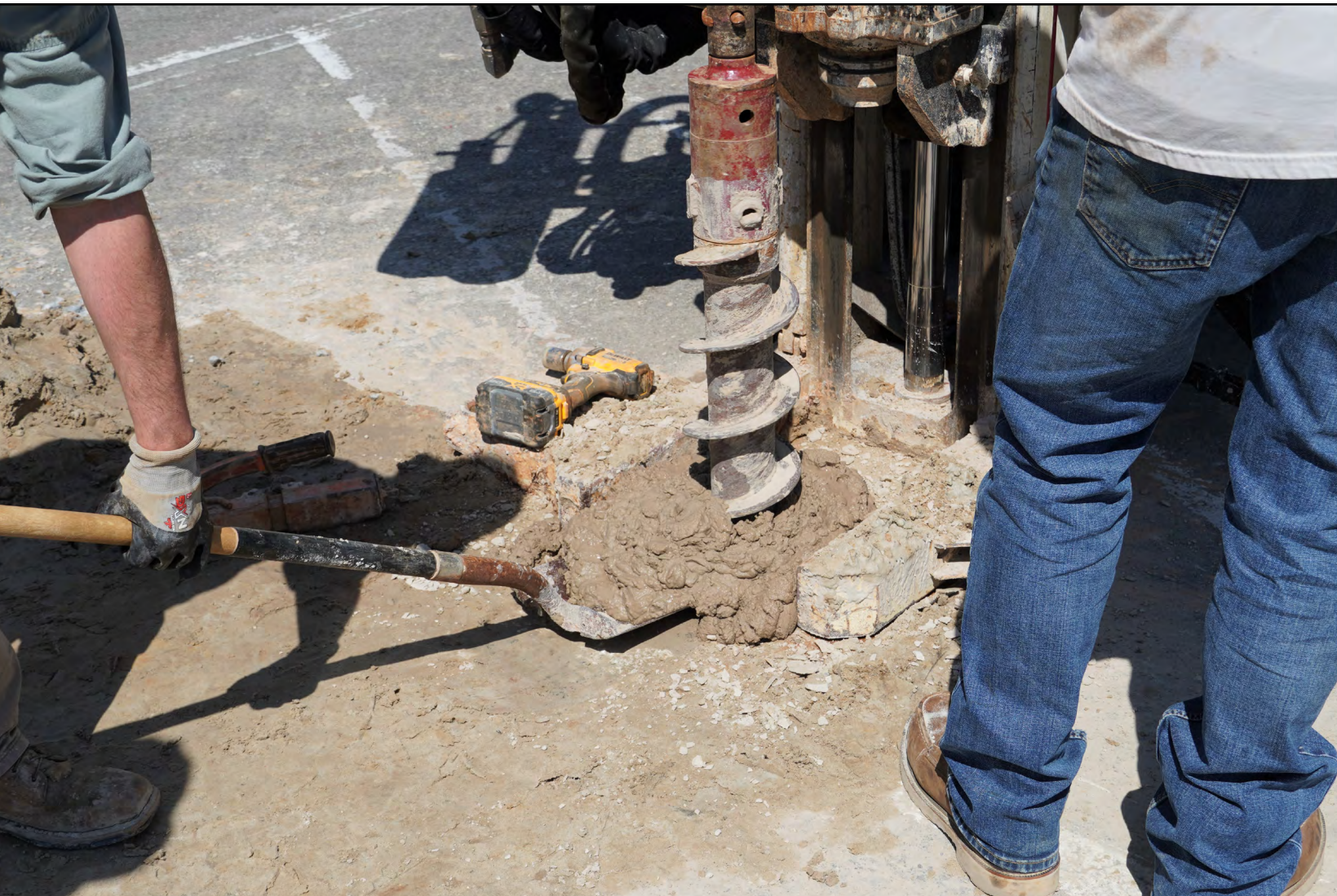
USACE Savannah District's geotechnical drill team began standard penetration tests at Hunter Army Airfield in Savannah, Georgia, to obtain soil samples March 13. The soil samples will provide critical data for future construction projects on the installation. (Photo by Michael Ariola)
