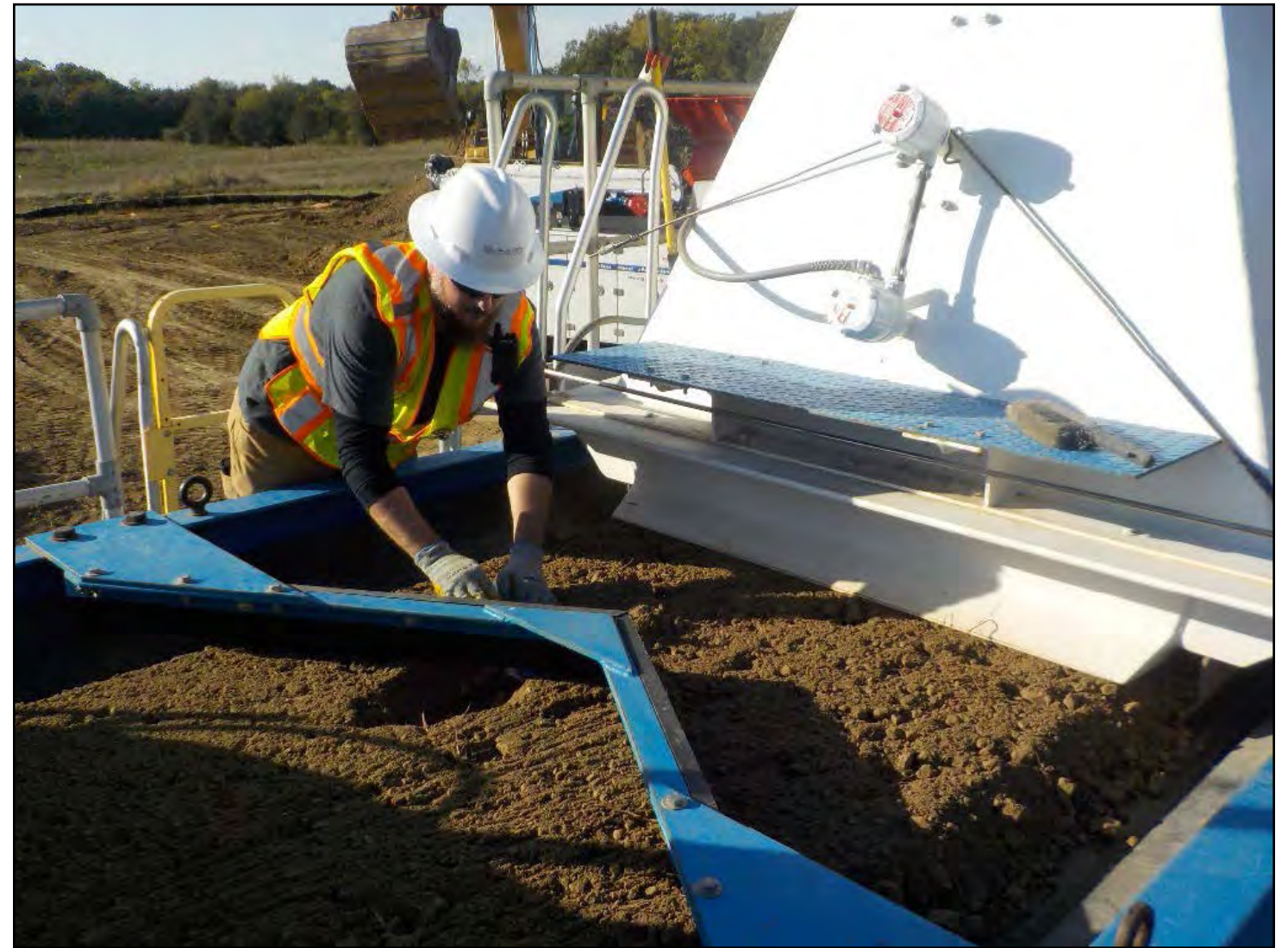
A contractor for the U.S. Army Corps of Engineers inspects the soil depth on the ISO-Pacific Soil Sorting System (S3). The S3 is an eco-friendly yet cost-effective way to identify and remove depleted-uranium radiological contamination in soil. (USACE Photo)
