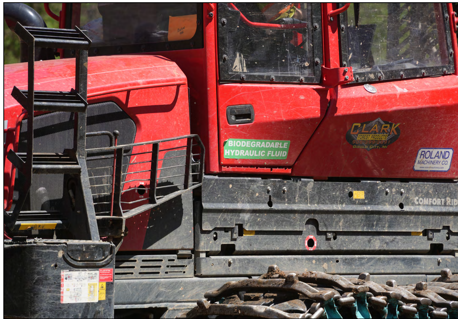
A "biodegradable hydraulic fluid" sticker is visible on a debris-removal vehicle operated by a USACE contractor April 15 along the Toe River in western North Carolina. The environmentally friendly fluid helps ensure that any potential hydraulic leaks do not harm the surrounding area as Hurricane Helene debris cleanup continues across the region. (Photo by Michael Davis).
