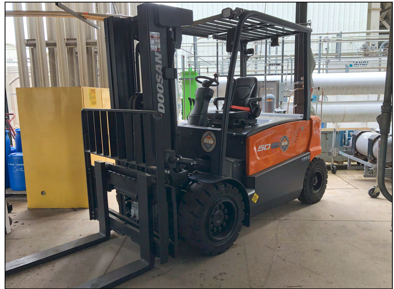
A hydrogen-powered fuel cell forklift was used during a demonstration at North Riverside Illinois Army National Guard as part of a larger research and development effort to integrate hydrogen energy solutions into military operations. (USACE Photo)
