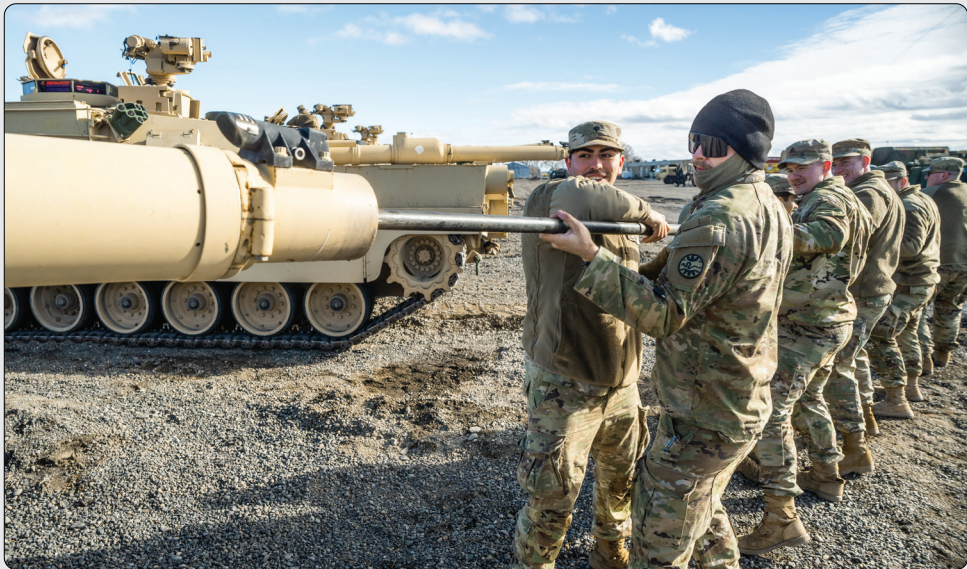
Tankers from Bravo Company, 3rd Battalion, 116th Cavalry Regiment, Oregon Army National Guard, conduct maintenance by cleaning the main gun tube of their M1A2 SEP v2 Abrams tank during an Inactive Duty Training weekend in Umatilla, Oregon, on Feb. 1, 2025.
