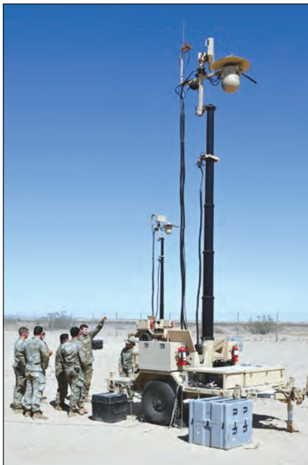
The Ground Based Operational Surveillance System (Expeditionary) is a multi-spectral sensor and persistent surveillance system that underwent developmental testing at Yuma Proving Ground in years past. (Photos by Mark Schauer)
