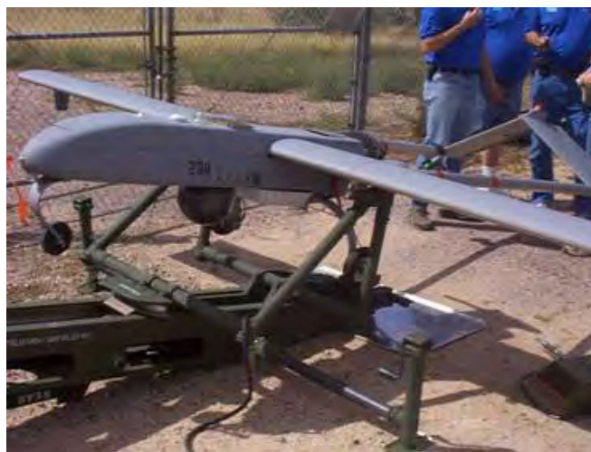
Photo 2-3. Shadow unmanned aerial vehicle launch.
