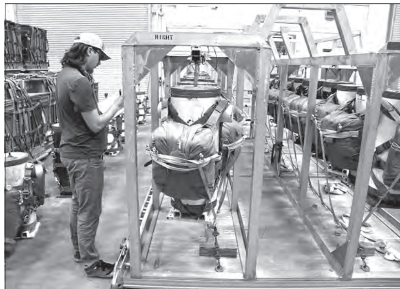
The T-11 personnel parachute offers jumpers a slow and stable descent, especially in high winds, and can support more weight than previous parachutes, a crucial advantage for warfighters who carry robust, heavy gear. Now long-fielded, the T-11 is still returning to Yuma Proving Ground for further refinements and improvements, including recently evaluated modifications to the corner vents. (Photo by Mark Schauer)
