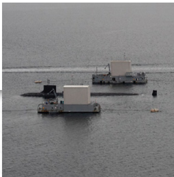
Full scale submarine acoustic signature measurements at our Southeast Alaska Acoustic Measurement facility
