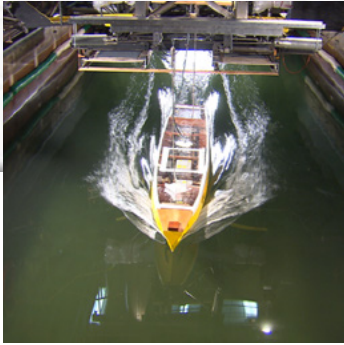
A model goes through a variety of seakeeping and propulsion tests in the David Taylor Model Basin
