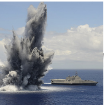
Full Ship Shock Trials (FSST) conducted on the LCS6 to validate operational survivability after exposure to underwater shock
