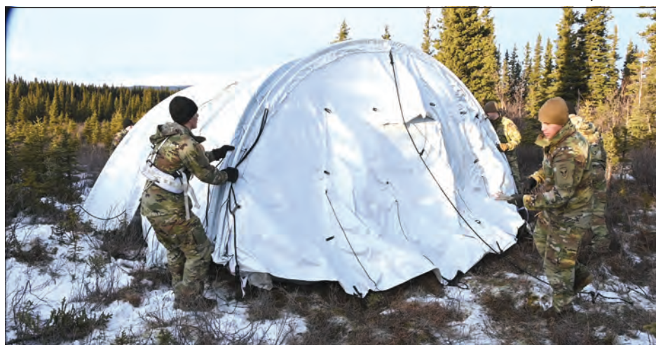
The Army’s Arctic Mobility Sustainment System (AMSS) and all-regions tactical clothing with updated cold weather clothing, snowshoes, and ski poles underwent rigorous testing at U.S. Army Arctic Regions Test Center (ARTC) this winter. The AMSS items under test will replace the legacy Ahkio sled and 10-person tent the Army currently uses.
