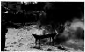
Mechanical foam is used on this oil fire, one of the many types of fires extinguished during week.
