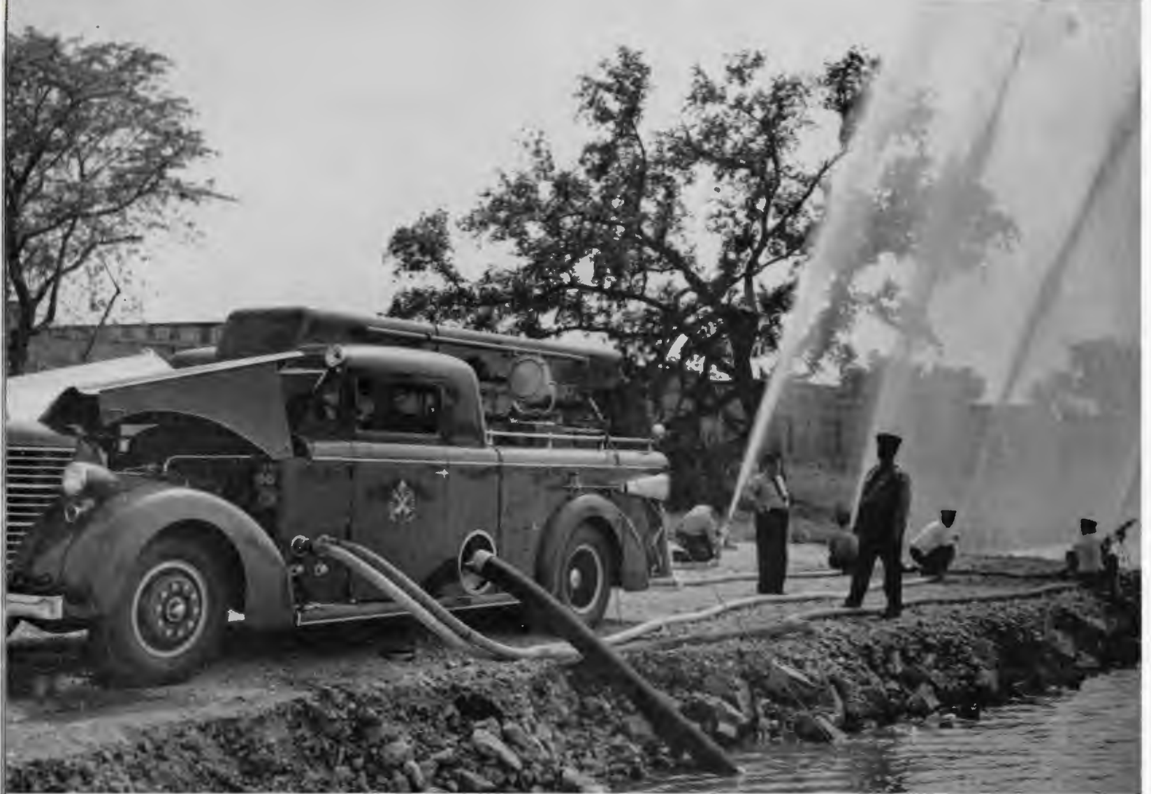
Arsenal pumper delivering pressure to four hose lines from intake in Mississippi. Pumper, in operation since 1941, can throw 1500 gallons per minute.
