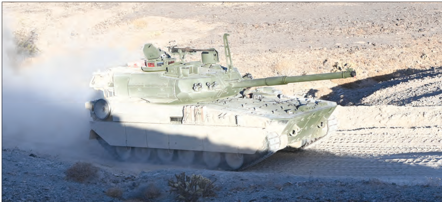
In addition to testing the armaments in both the natural environment and from a cold chamber, the platform is subjected to a full complement of performance and reliability, accessibility, and maintainability testing. Test vehicles are running across punishing desert road courses, up steep slopes and through a watery fording basin, sometimes while under a full load.
