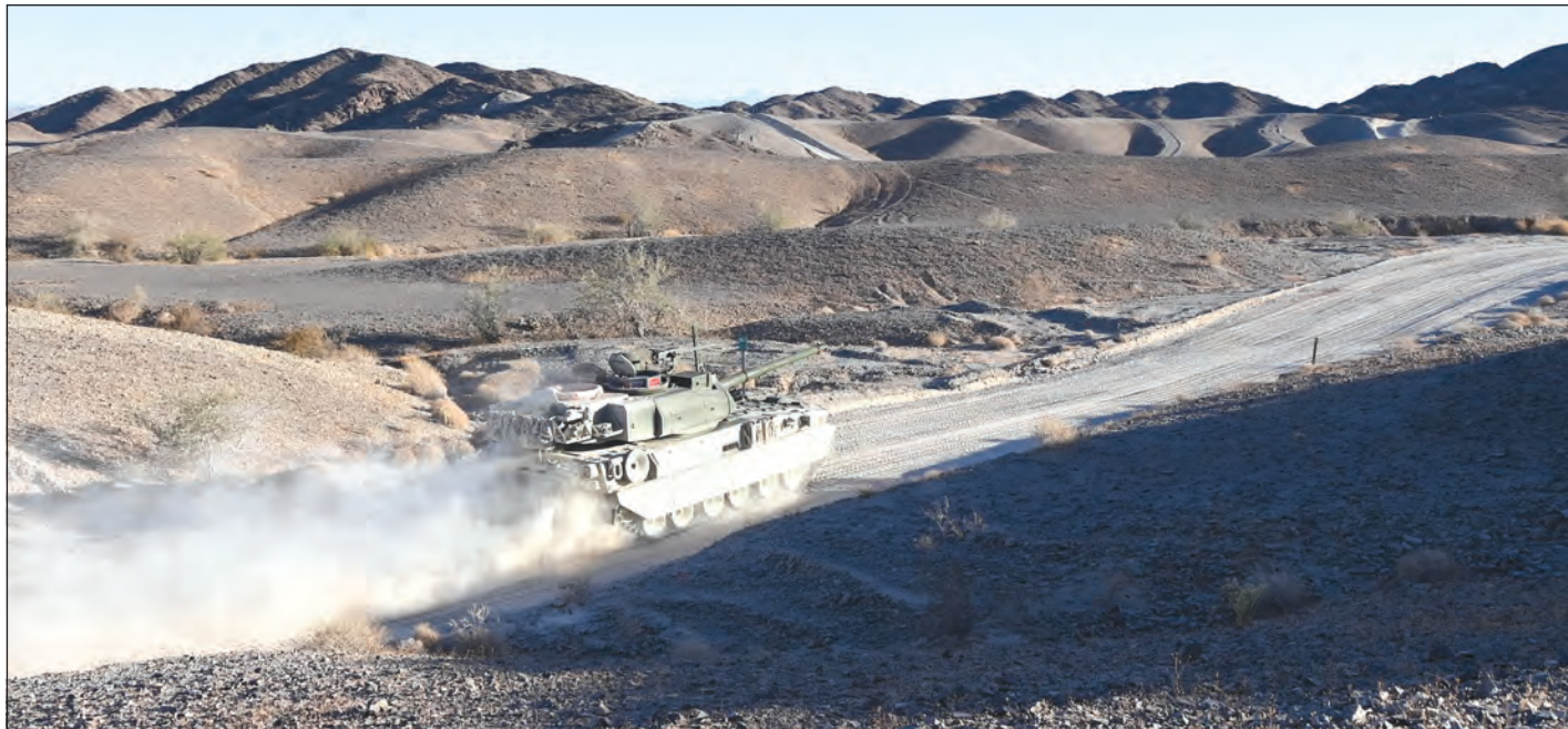
The M10’s main weapon is a M35 105mm low-recoil tank gun, significantly larger than the 25mm chain gun on the Bradley and boasts a 12.7mm M2 heavy machine gun and 7.62 mm Coax machine gun. The platform’s diesel engine puts out 800 horsepower and can power it up to 40 miles per hour. (Photos by Mark Schauer)
