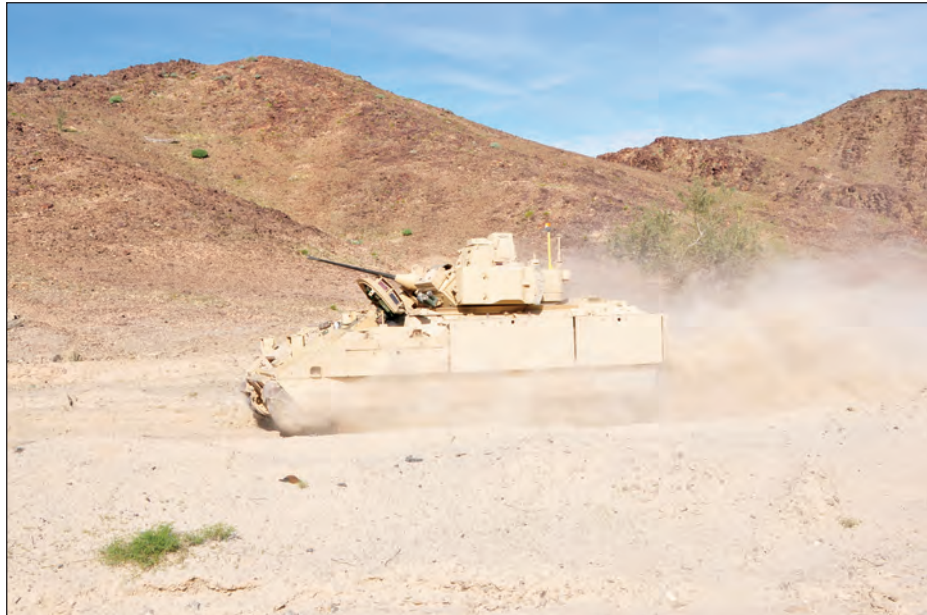
Recently, U.S. Army Yuma Proving Ground personnel conducted a production qualification test on the Vehicle Protection System Base Kit (VBK) of the Bradley Fighting Vehicle, which utilizes sensors on the corners of the turret to provide 360 degrees of detection for incoming laser threats. (Photo by Mark Schauer)
