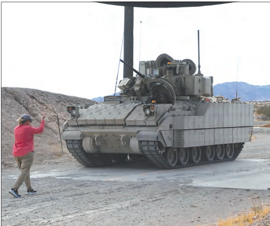
LEFT: During testing, simulated missions took the Bradley 6,500 miles across Yuma Proving Ground road courses featuring various terrain conditions, from paved to gravel to punishing desert washboard that would severely rattle less robust vehicles. RIGHT: The Bradley Fighting Vehicle has proved itself to be lethal and survivable in multiple theaters since first fielded in the 1980s. (Photos by Mark Schauer)
