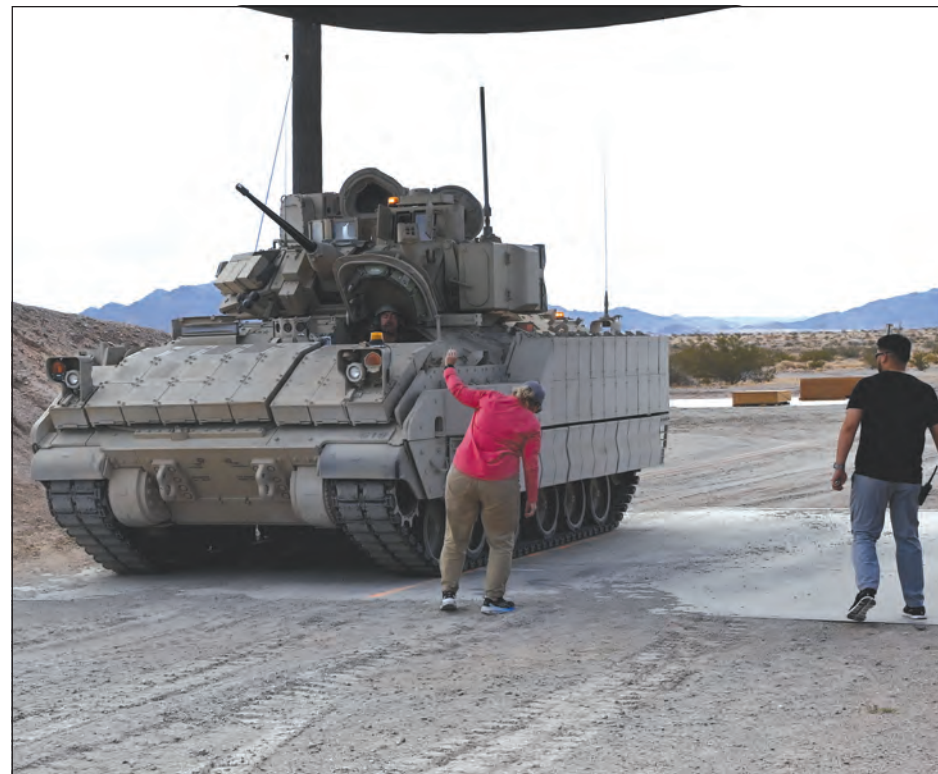
LEFT: During testing, simulated missions took the Bradley 6,500 miles across Yuma Proving Ground road courses featuring various terrain conditions, from paved to gravel to punishing desert washboard that would severely rattle less robust vehicles. RIGHT: The Bradley Fighting Vehicle has proved itself to be lethal and survivable in multiple theaters since first fielded in the 1980s. (Photos by Mark Schauer)
