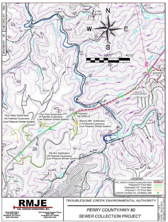
Figure 1. USACE funding design and construction area of the proposed Perry County/HWY 80 Collection Project Phase III, Knott and Perry counties, Kentucky (Source: RMJE 2022).
