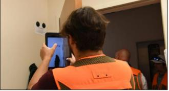
Aug. 19, 2024: An environmental specialist at Naval Support Activity (NSA) Naples, Italy, affix detectors in buildings as part of Radon testing of non-residential rooms, buildings and unaccompanied residences. Radon is a colorless, odorless, tasteless gas that is produced by the breakdown (radioactive decay) of naturally occurring uranium found in rock, soil, and water.
