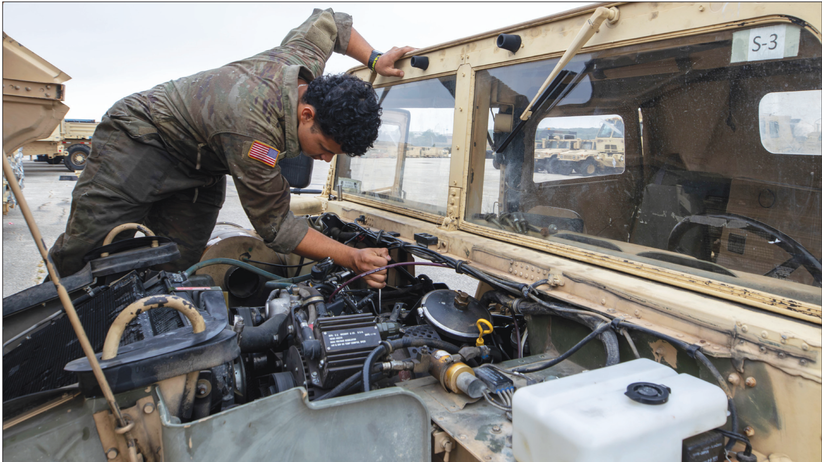
Photo by 1st Lt. Russell Shirley-Jones, III Armored Corps Public Affairs Pfc. Stiven Ramirez, wheeled vehicle mechanic, Echo Company, 1st Battalion, 227th Aviation Regiment, 1st Air Cavalry Brigade, connects the fuel pump line on a M1097R1 High-Mobility Multipurpose Wheeled Vehicle, or HMMWV, Nov. 7 at Fort Cavazos.
