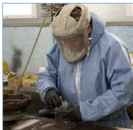
Maintenance personnel wearing personal protective equipment (PPE) required to protect against Cr(VI). Photo provided by the authors.
