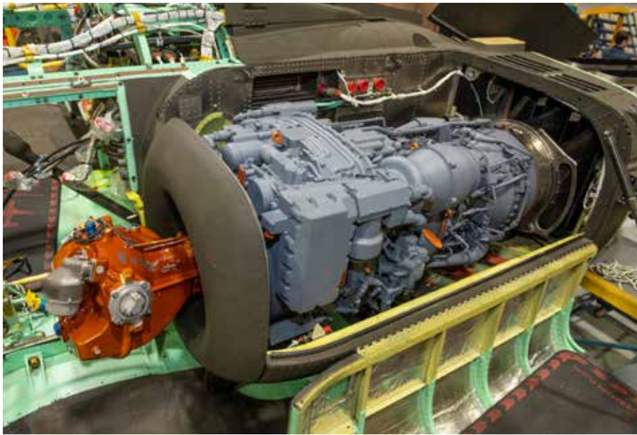
The Additively Manufactured (AM) 3D model of the T901 engine, shown installed in the engine bay of an Apache AH-64E helicopter for fit testing. Photo by Paul Stevenson, PEO, Aviation.
