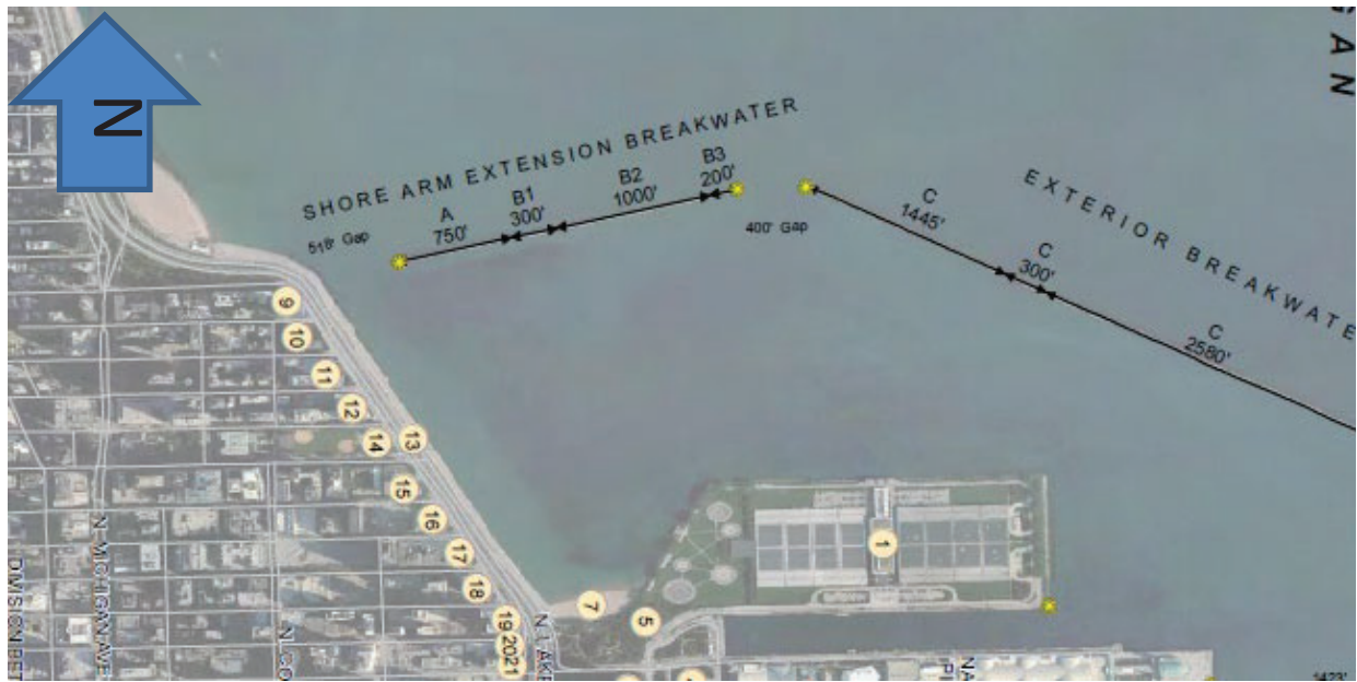
Figure 4. Chicago Harbor Shorearm Extension Breakwater intended work, intended work depicted by orange arrow (adapted from previous contract documents)
