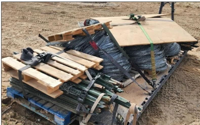
Figure 1 — Example of a Poorly Built Combat Configured Load Packed with Concertina Wire, Pickets, and Barbed Wire (Note the concertina wire falling over and randomly placed ratchet straps.)
