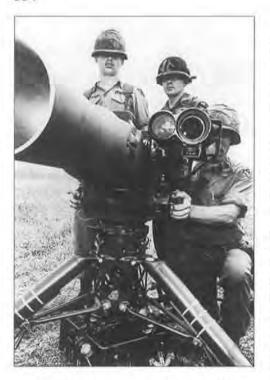
TOW (tube-launched, optically tracked, wire-guided) missile
