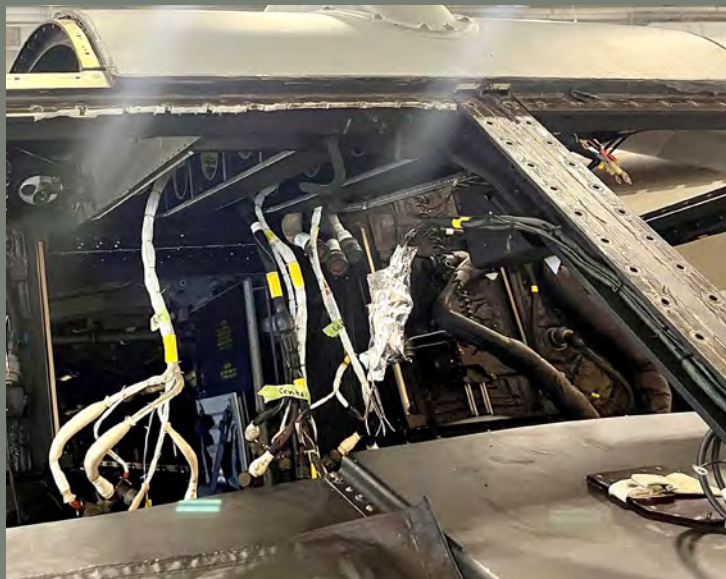
Aircraft ready for structural repair. Note the top shear line through the screw holes where the support structure failed.
