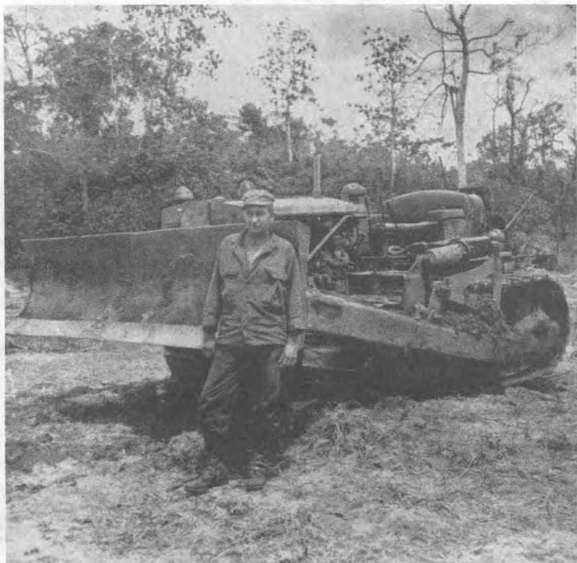
D-7 BULLDOZER operated by Private Webster J. Ough, Troop C, 8th Engineer Squadron, enabled tanks to move through the jungle to Number One Road. Bulldozers were also used extensively to demolish bunkers.
