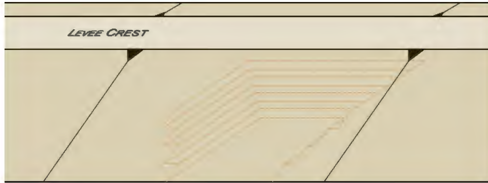
Figure 5: The excavation is backfilled and trimmed to allow topsoil placement to the design slope.
