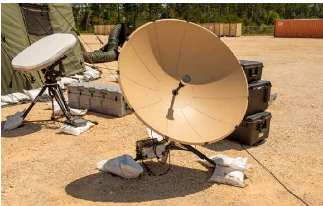
NETC2 equipment demonstrated at the Waterside Symposium: front and center (tan), a Hawkeye 4 Lite satellite terminal, back, left (white) a Copasat Storm satellite terminal.
