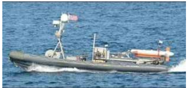
Mine Hunting Unit (MHU) Unmanned Surface Vehicle in transit with an AQS-24 mine hunting sonar.
