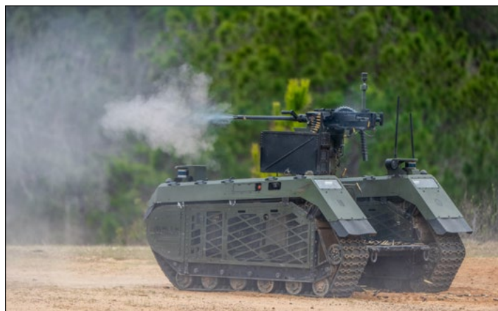
The Milrem THeMIS, a Dutch and German ground-based system combining an unmanned ground vehicle and a remote-controlled weapon station, participates in the 2024 AEWE on 29 January.
