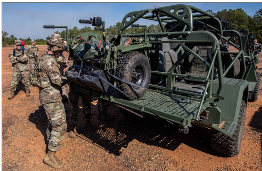
Technology and industry leaders unload and set-up their concepts to demonstrate their submissions on 2 February 2024 at Fort Moore, GA. The Silent Tactical Energy Enhanced Dismount is an all-terrain, electric payload mobility platform which is tactically silent and has zero emissions. (Photos by Patrick A. Albright)
