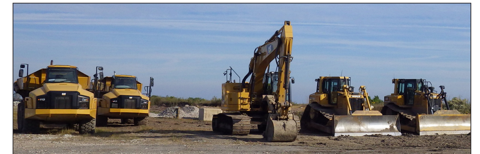
Dump trucks ( left ), excavator ( middle ), and bulldozers ( right )
