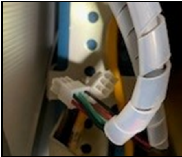
Connect battery harness to fusible link connector
