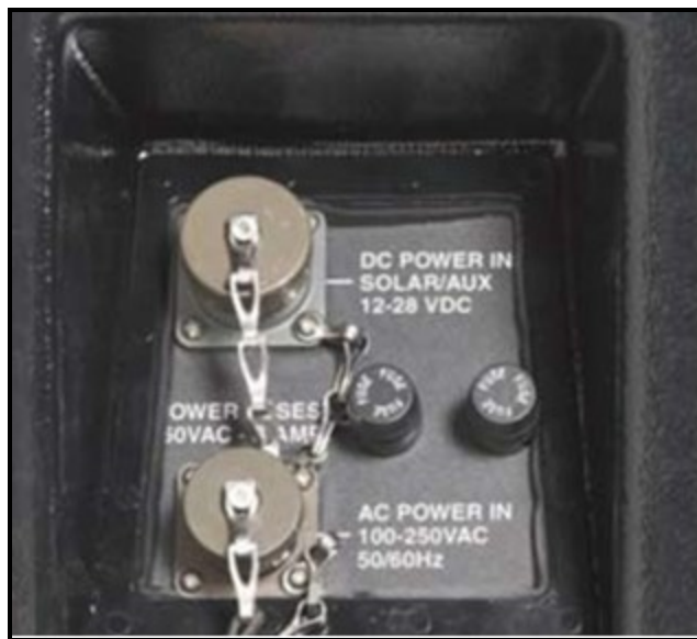
Connect AC power cord to ECU power panel
