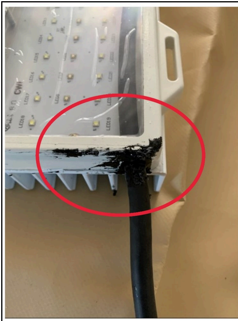
Damage caused by defective rubber grommet
