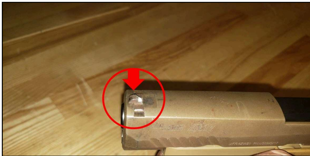
Adjusting the front sight on the M17/M18 pistol can lead to damage
