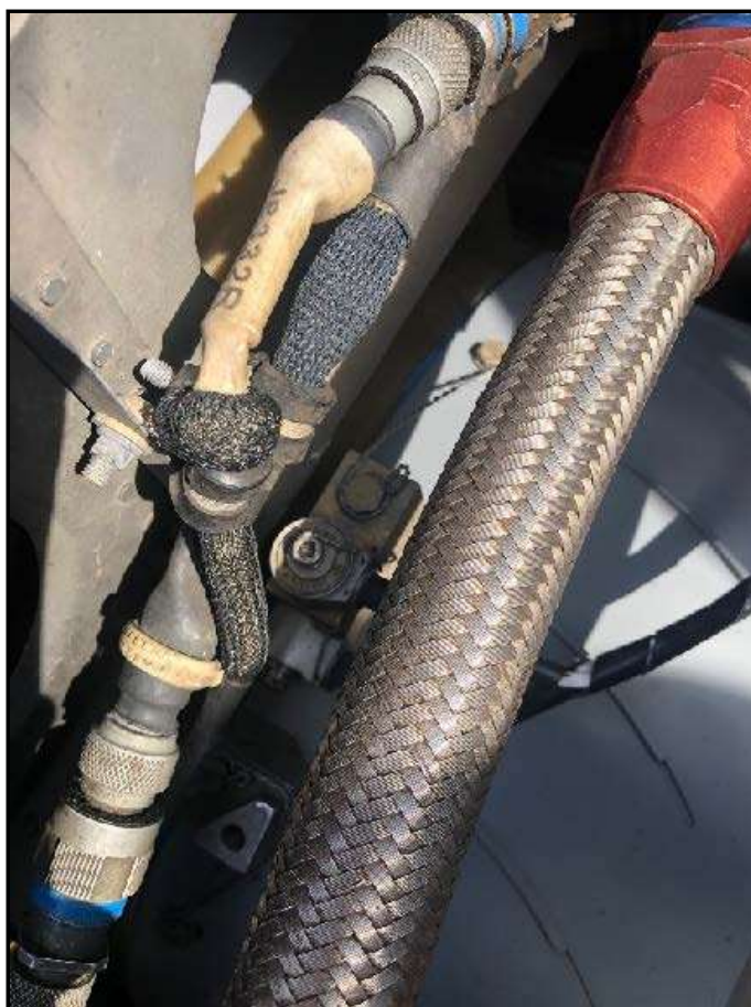
Oil cooler sensor mounting block installed incorrectly
