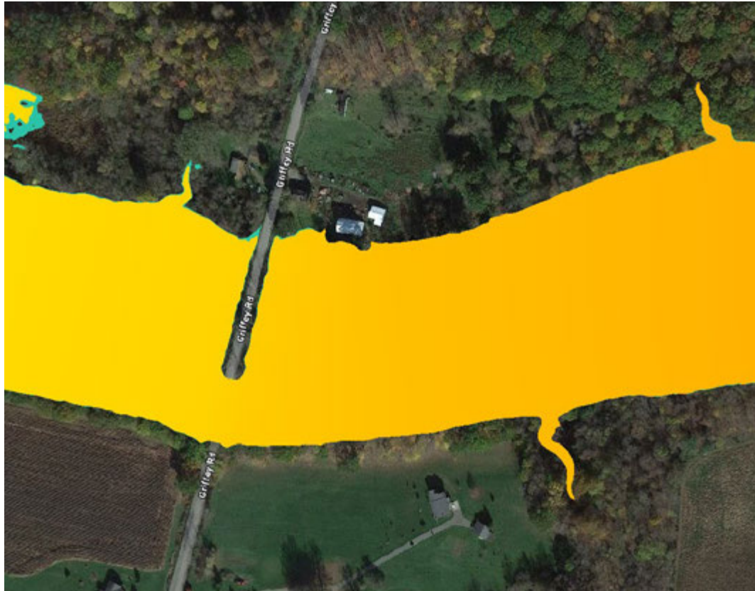
Figure 14. 0.2% ACE Inundation Boundaries for Recommended Manning's n Values (Orange) to Maximum Manning's n Values (Blue)
