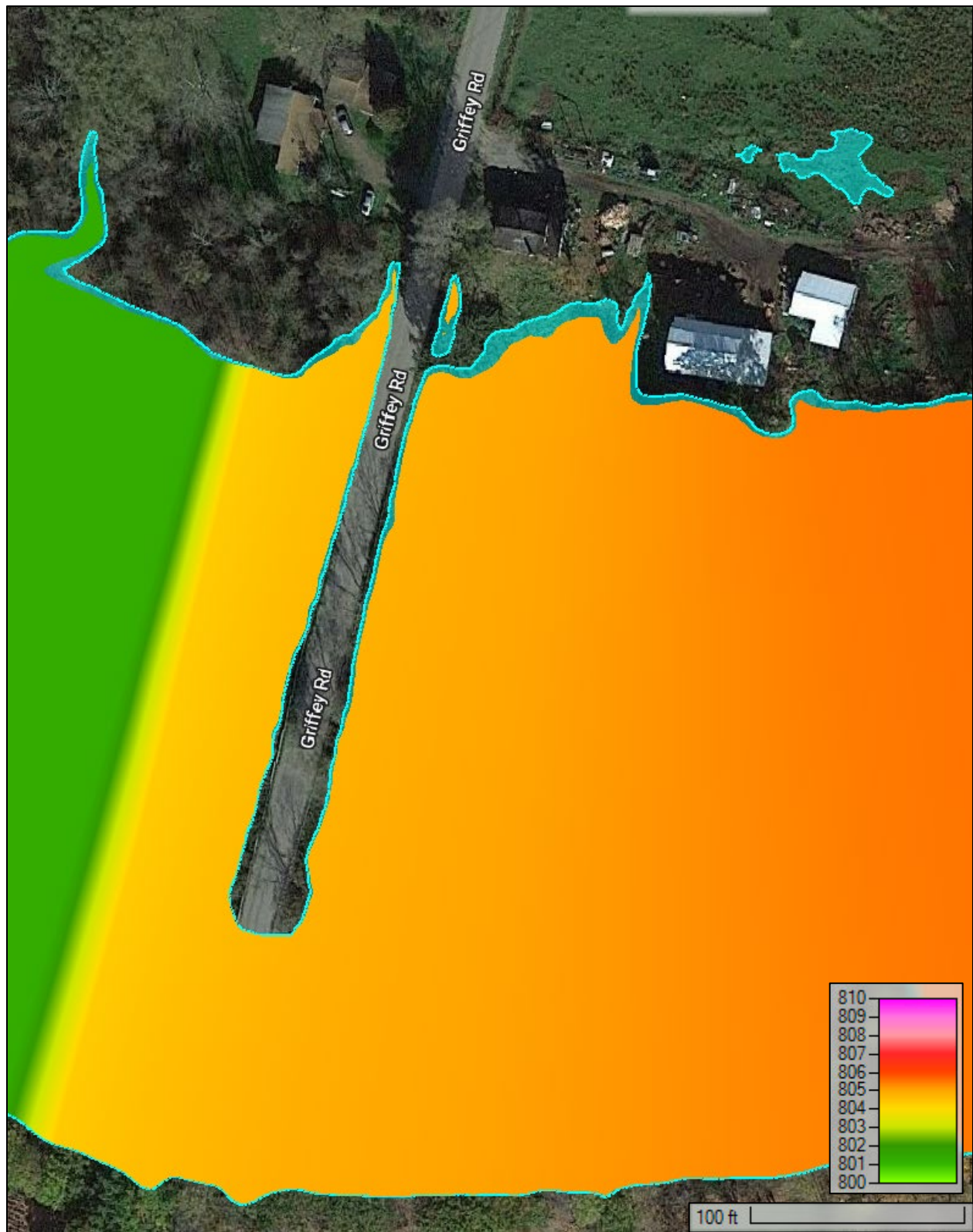
Figure 51. Parcel D Structures Footprints Outside of the 1% ACE TSP Barrier WSE (Orange-Green Gradient) and 0.2% ACE Inundation Extent (Cyan)
