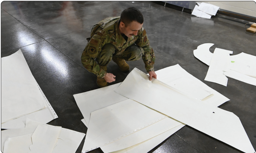
ORANG Staff Sgt. Drew Sorlien, a structural maintenance technician with the 173rd Maintenance Squadron, organizes the Kingsley Field eagle tail flash stencils before placement on the F-15C begins, Jan. 17, 2024, at Kingsley Field. Painting the tail flash requires several layers of stencils that must be done in the correct order.
