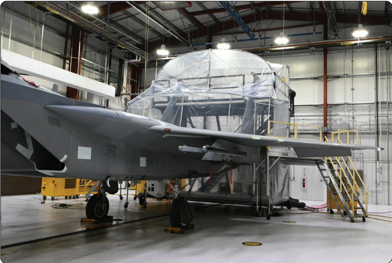
Airmen from the 173rd Fighter Wing structural maintenance section construct a custom PVC pipe frame enclosing the tail of the F-15C requiring paint, Jan. 17, 2024, at Kingsley Field in Klamath Falls, Oregon.
