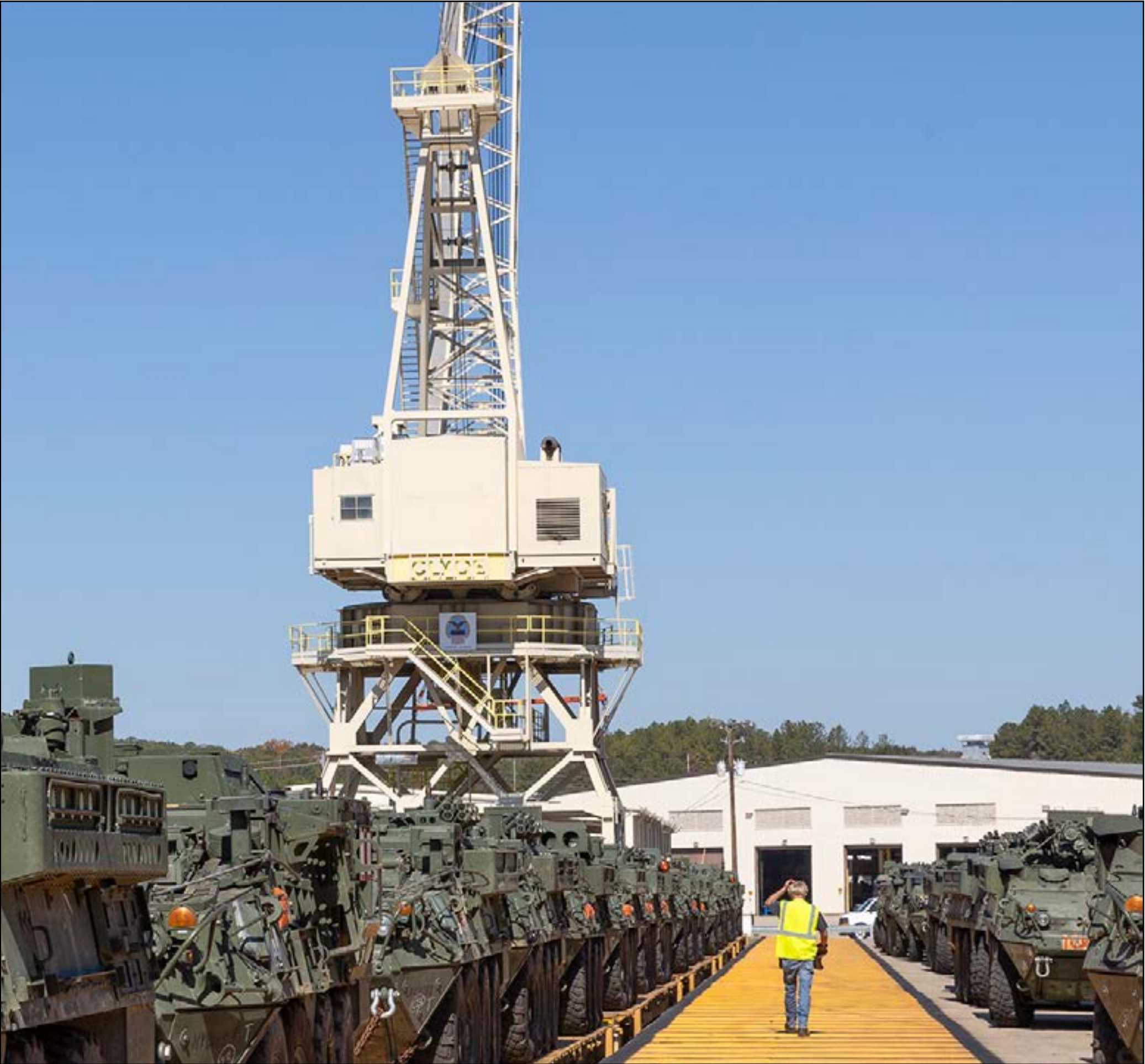
A $2.7 million refurbishment and modernization project upgraded Clyde’s original lift capacity from 75 tons to 80 tons, enabling crews to load and unload over 100 train cars each carrying two M1 tanks.
