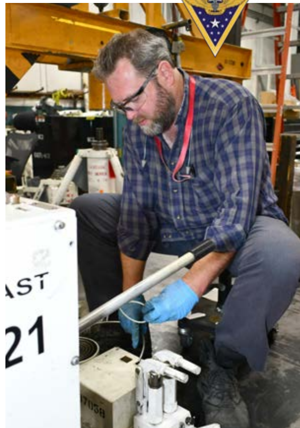
Beary Spear, powered support systems mechanic in the Fleet Readiness Center East (FRCE) ground support shop, drains fluid from an aircraft jack. This year, mechanics in the Ground Support Branch are scheduled to perform more than 5,000 preventive maintenance operations on more than 2,000 items of equipment. Mechanics check bearings, change fluids and perform other maintenance operations, as well as any necessary repairs to safety stands, powered test and transportation equipment and electric carts.
