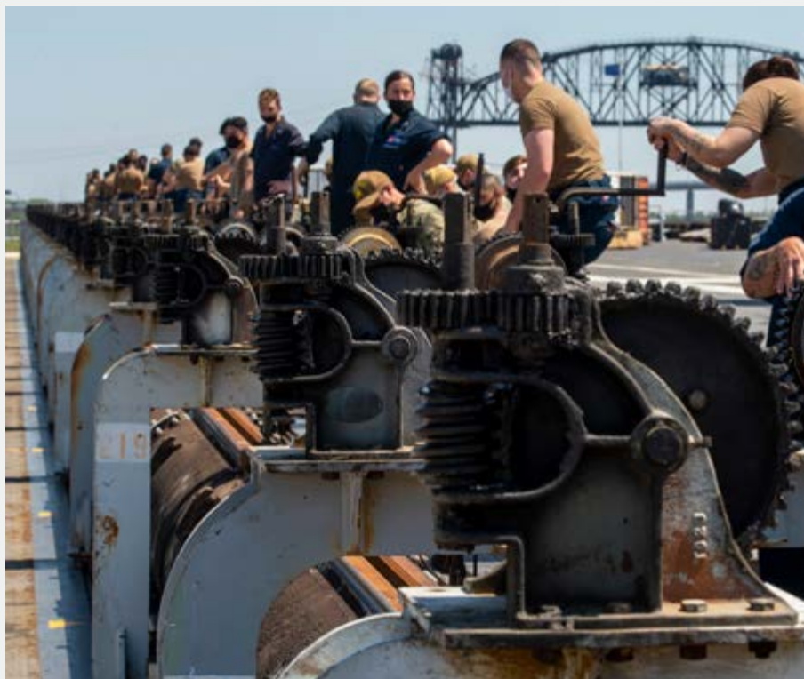
Sailors conduct catapult maintenance on the flight deck aboard aircraft carrier USS George H. W. Bush (CVN 77).
