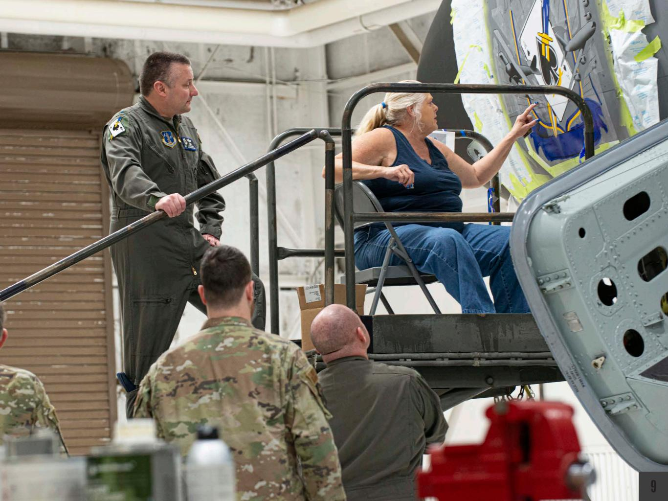
Aero repair was brought in to bring down the tail and remove the rudder. They brought the rudder into the Fuel Cell hangar to be primed and then painted. Approximately four large SUVs worth of paint was used to paint the entire tail..
