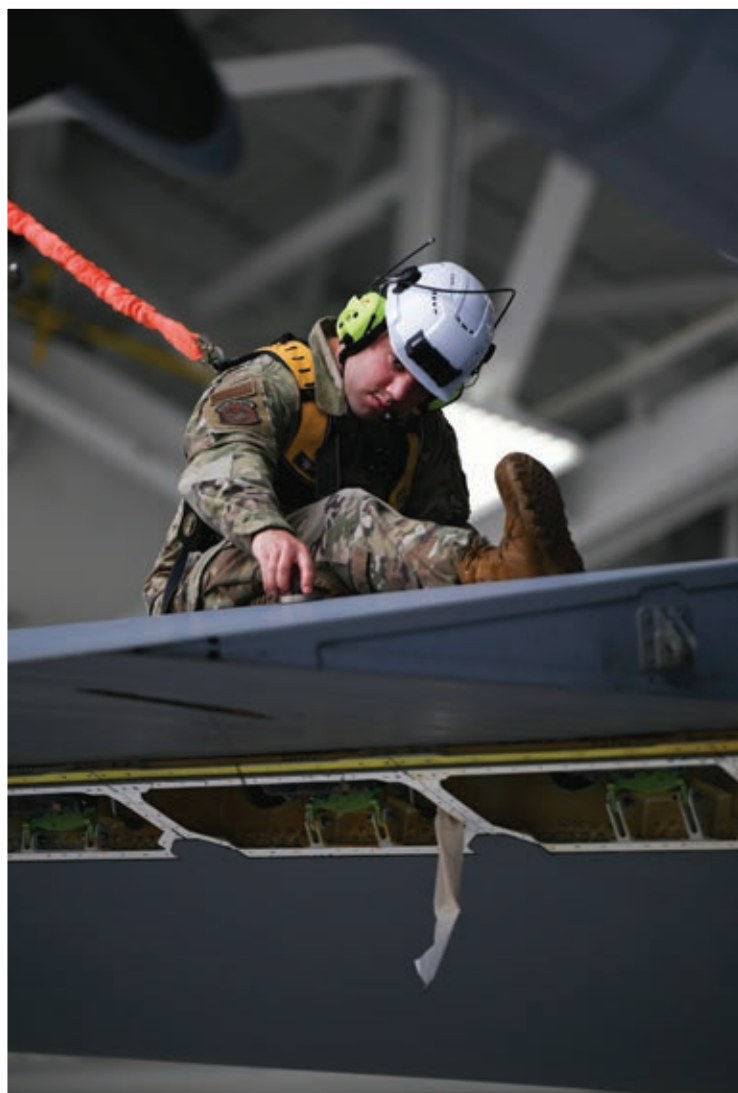
Tech. Sgt. William Rand , an aircraft maintainer with the 157th Maintenance Group, coordinates the removal of the flight control surface with the maintenance team and equipment operators Oct. 5 at Pease Air National Guard Base in Newington.
