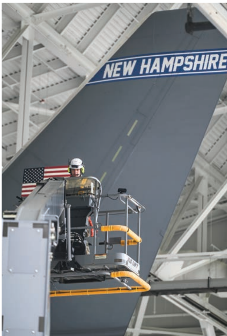
Tech. Sgt. William Rand , an aircraft maintainer with the 157th Maintenance Group, coordinates the removal of the flight control surface with the maintenance team and equipment operators Oct. 5 at Pease Air National Guard Base in Newington.
