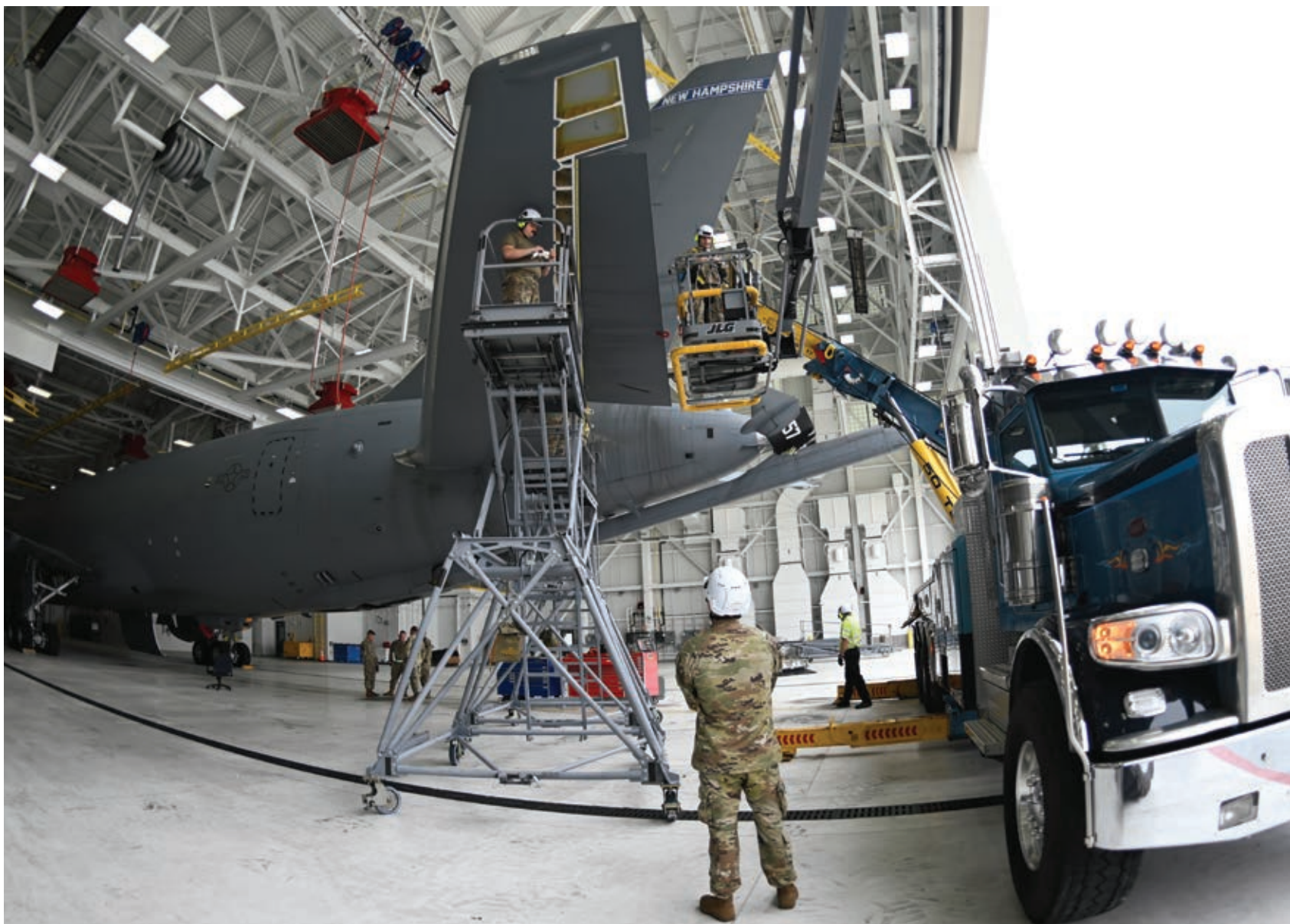
Airmen of the 157th Maintenance Group and 64th Air Refueling Squadron replace an elevator on a KC-46A Pegasus on Oct. 5 at Pease Air National Guard Base in Newington.
