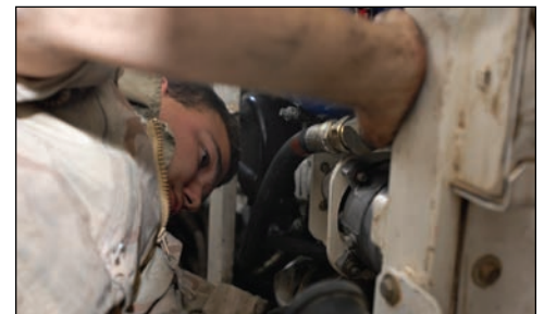
Pfc. Jeff Basile, a mechanic with 1st Combat Repair Team, Company B, 702nd Brigade Support Battalion, squeezes into the driver's hull of a Stryker to carefully attach the fuel, air and hydraulic hoses to a Stryker engine here May 20.
