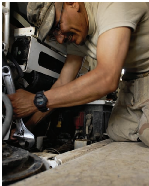
Spc. Angel Hernandez, a mechanic with 1st Combat Repair Team, Company B, 702nd Brigade Support Battalion, fixes a nitrogen pump to the inside of a Stryker, here May 20 to fill the vehicle's nitrogen tanks.
